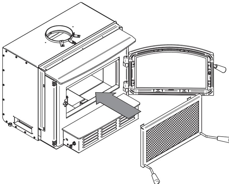
3. Lean the upper part of the fire screen against the top door opening making sure to insert the top fire screen brackets behind the primary air deflector.
