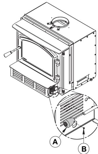
Figure 24 : Installing the air control wood handle
