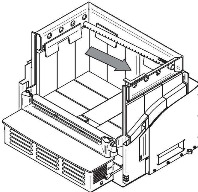
2. Align the notch in the left end of the tube with the key of the left air channel hole. Using a « Wise grip » hold the tube and lock it in place by turning the tube as shown. Make sure the notch reaches the end of the key way.
