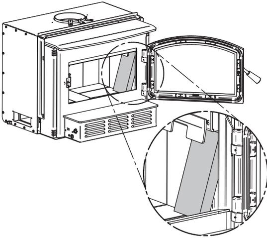
Figure 25 : Install the Combustion Chamber Bricks
