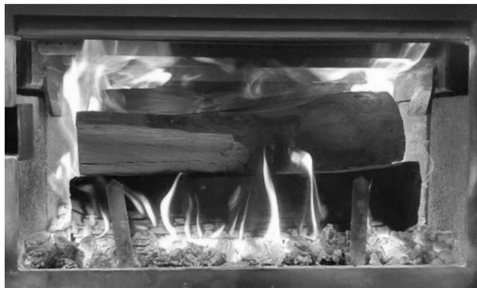
Close the primary air control by small increments (ex: 1/16 of an inch), from ½” to fully closed, between 4 and 15 minutes after the loading period. Before closing further, make sure the flame intensity is increasing or stable. Close the air control completely. Turn ON the blower at maximum speed.
