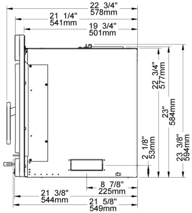
Figure 4 : Side View - Maximum Insert Projection
