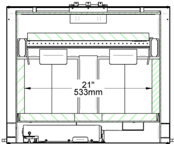
Figure 6 : Front View - Combustion Chamber
