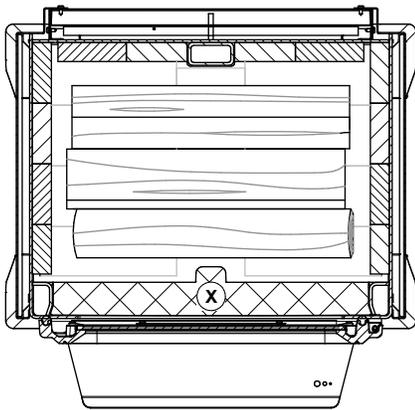
Figure 11: Position of the bottom pieces (High burn)
