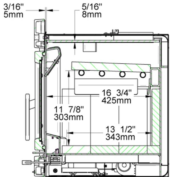
Figure 7 : Side View - Combustion Chamber
