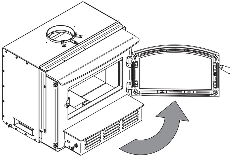
2. Hold the fire screen by the two handles and bring it close to the door opening.
