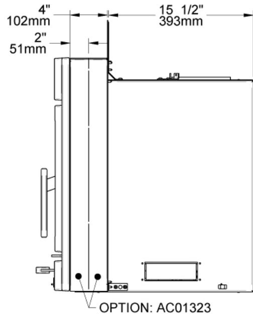
Figure 2 : Side View - Minimum Insert Projection
