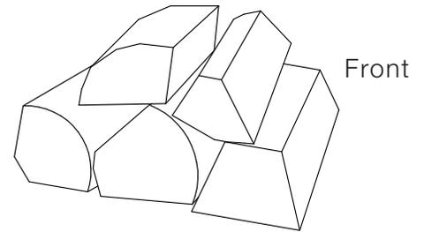
Figure 19: Example medium burn load (side view)
