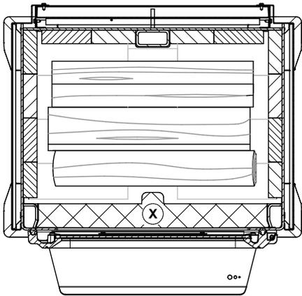
Figure 17: Position of the bottom pieces (Medium burn)
