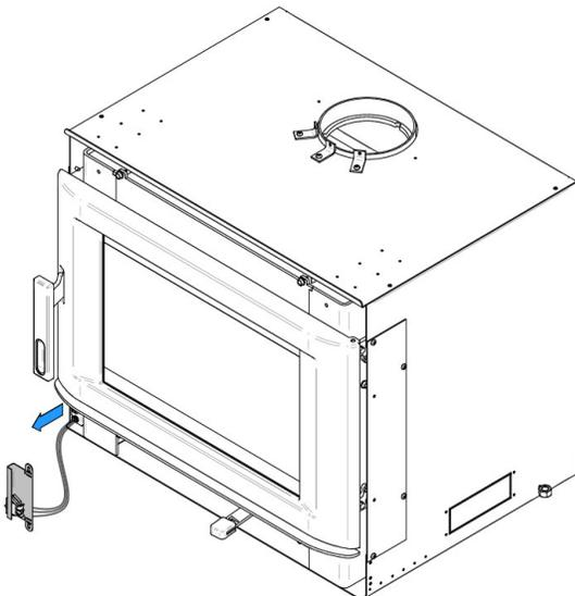
4. Approach the faceplate and screw the blower switch assembly on the left hand side.
