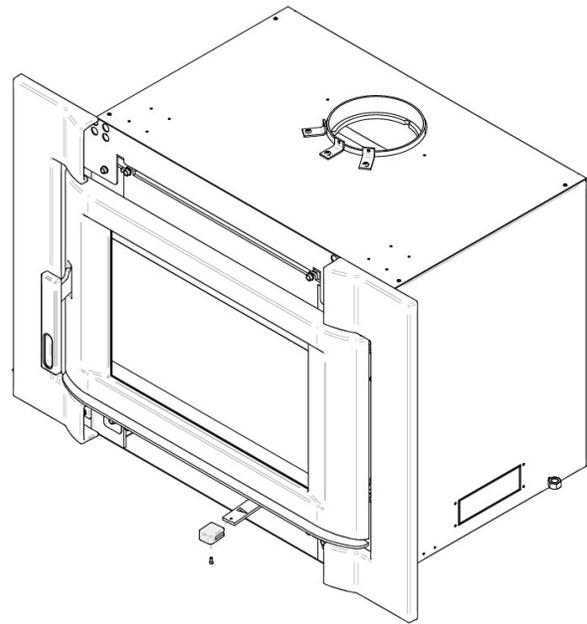
7. Slightly unscrew the two screws at the bottom of the insert. Hook the bottom faceplate and screw it back in place. Reinstall the wood handle.
