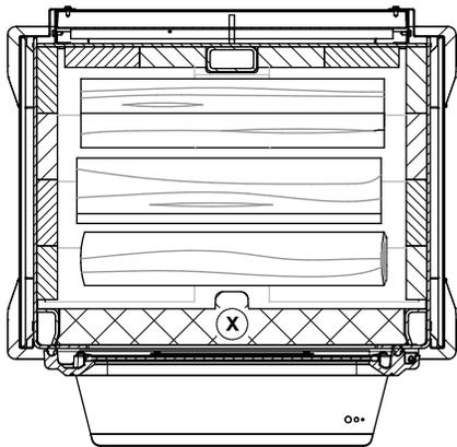
Figure 14: Position of the bottom pieces (Low burn)
