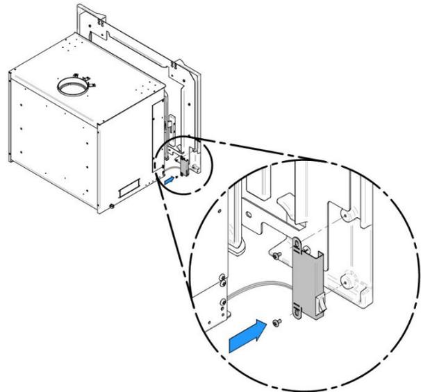
5. Install the faceplate on the insert, being careful not to pinch the blower switch wires.
